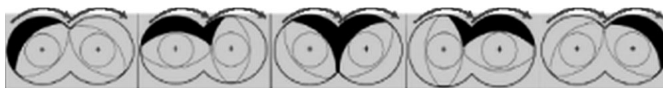
Figure 1 Material flow through an intermeshing corotating twin-screw extruder.
